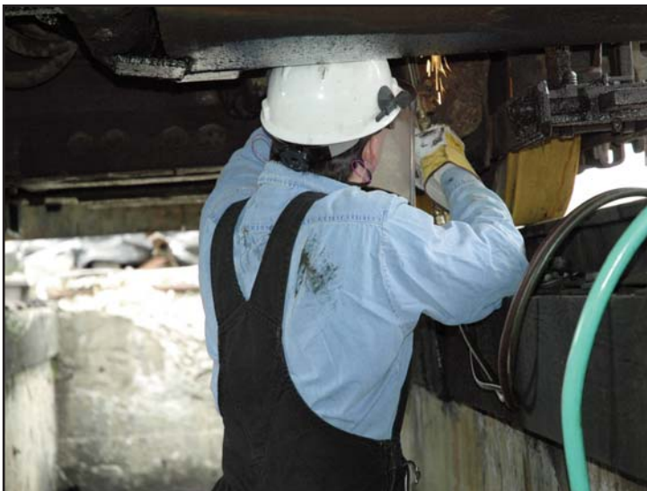
Dan Carleton was in a railyard pit, working over his head to remove a traction motor gear case from the SW-8 Pfizer locomotive during December. Photo by Geoff Knees.
